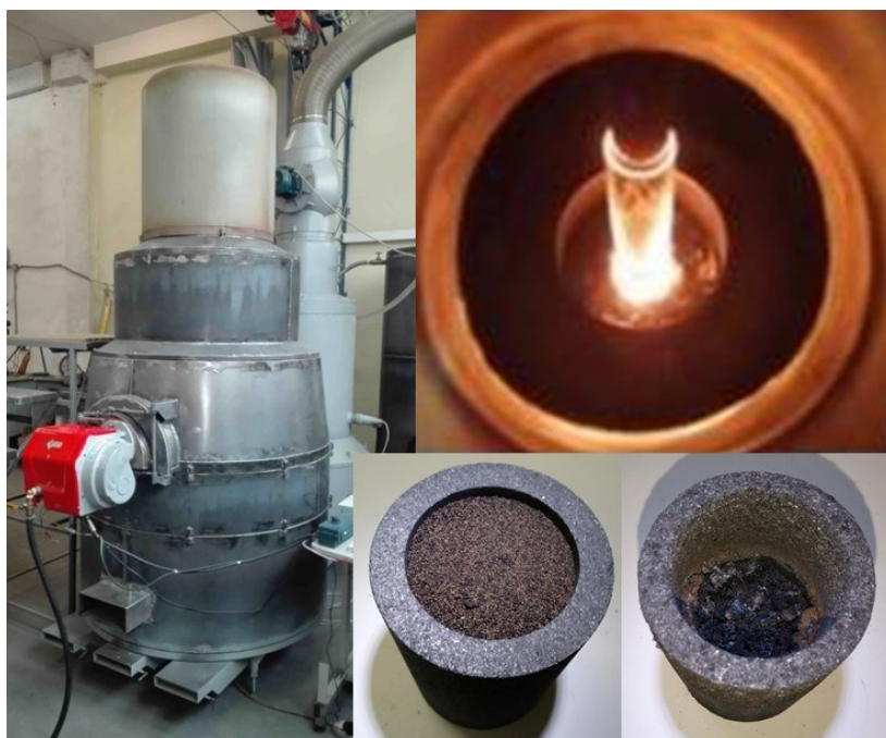
Figure 10. The pilot scale gasifier for the treatment of Ion Exchange Resins (SIIEG).
