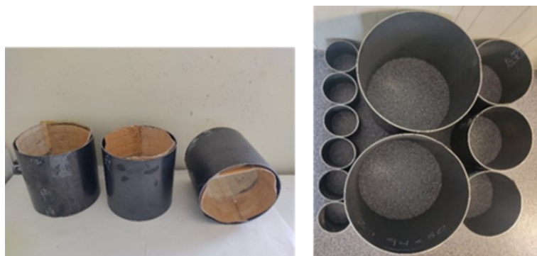
Figure 7. Metallic pipes contaminated with Cs-137 ready for non-destructive gamma spectrometry measurements (NCSR, Greece).
