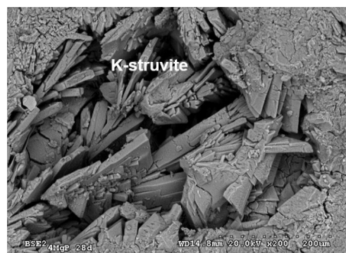
Figure 8. Magnesium phosphate cements prepared using excess of Mg to phosphate and volcanic ash as filler showing crystals of K-struvite: ( KMgPO_4 \cdot 6H_2O ) (UAM, Spain).
