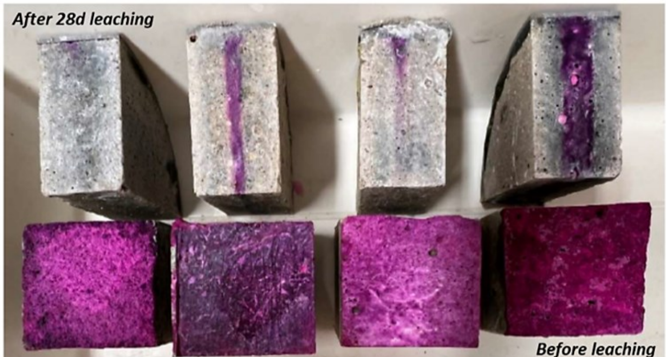
Figure 9. Leaching experiments for four composites: AAM/oil. The chemical formulation of the AAM vary especially the w/s ratio. 20-25% vol of Nevastane or Shell mineral oil is stabilized in the activated binder. Task 5.4.4
