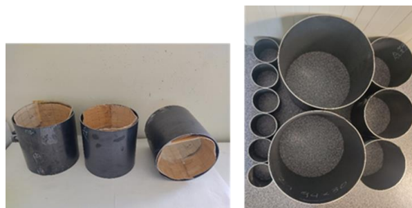
FIGURE 8. METALLIC PIPES WITH DIFFERENT DIMENSIONS TESTED FOR THE OPTIMISATION OF THE NDC GAMMA SPECTROMETRY TECHNIQUE.
