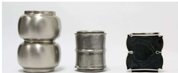
Figure 7 Synroc® container before and after HIP treatment (Image: ANSTO)
