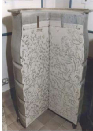
Figure 2 Blocking in cement of Magnox fuel cladding swarf (Image: Savannah River National Laboratory).
